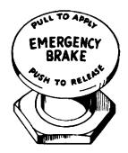
An emergency brake control is **located in the upperstructure cab.** This control is to be used in case of failure of the automatic digging brake. If digging brake fails to apply when travel pedal is released, raise emergency brake control to apply emergency brake. Notify maintenance personnel immediately for repair of digging brakes.
