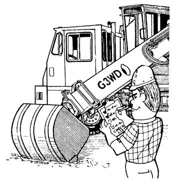
Maintain three point contact with grab handles and steps when climbing on and off the machine. Never jump from the machine.
